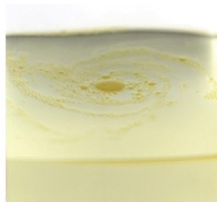
Ninhydrin Working Solution with 'oily' droplets floating on the surface.
