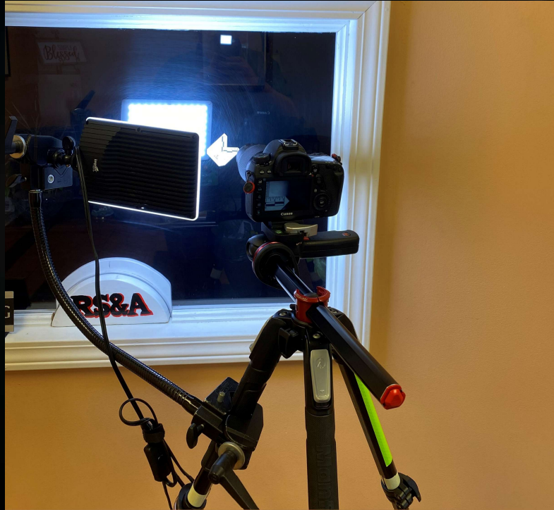
Camera and tripod setup for photographing unprocessed latent print on window
